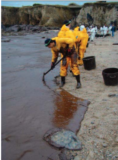
Figure 5-14: Nile Blend crude (pour point +33°C) in sea water of 28°C [ITOPF; 2005]
