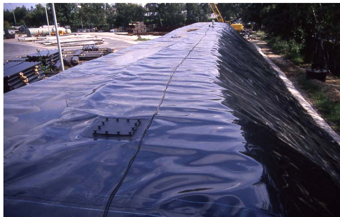
Figure 5-32: Cover of foil on a windrow protected against rain, erosion and evaporation
