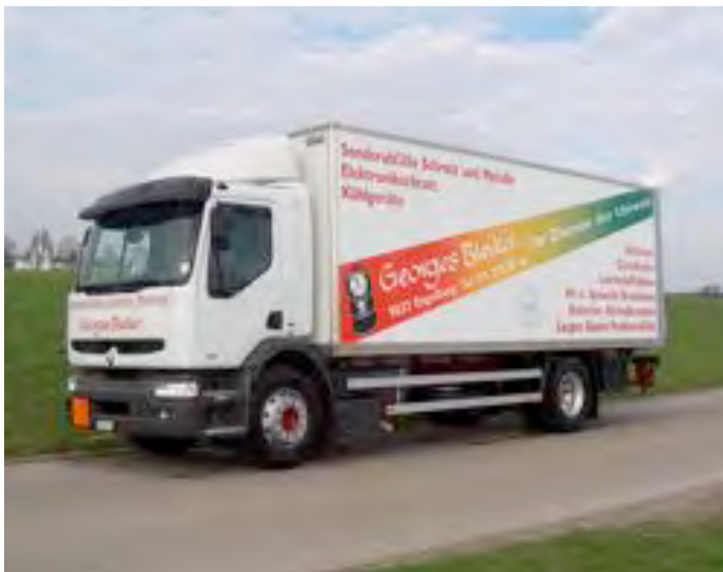
Figure 4.5-2: Special truck for the collection of hazardous household waste [Bleiker GmbH, 2007]
