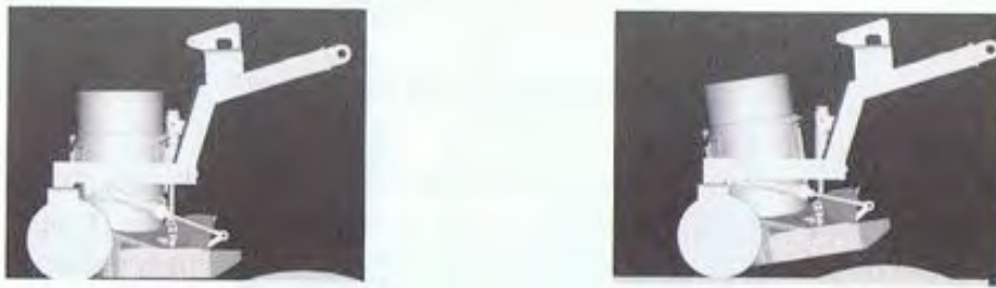
Figure 4.3-4: Attachment to clean (for example) speed bumps in traffic calmed area 32
