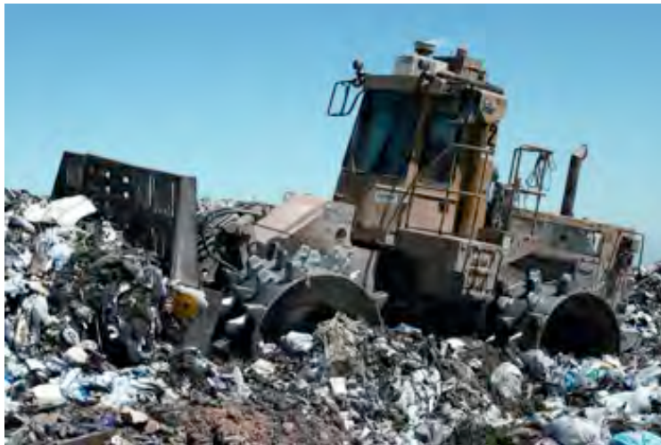
Figure 5.6-15 Landfill compactation [image on public domain]
