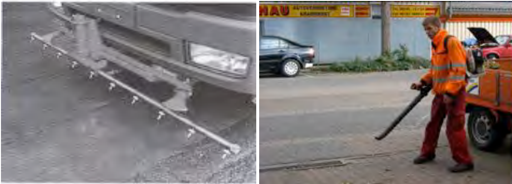
Figure 4.3-6: Machine with special sprays to clean below parking cars (left) 35 , leaf blower (right) 36
