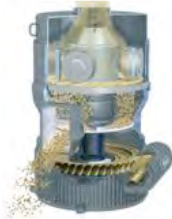
Figure 5.2-9: Principle of a pellet press [Kahl, 2007]
