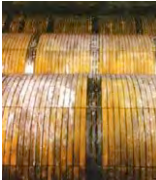
Figure 5.4-4: Rotary drum grate [Igelbüscher, 2005]
