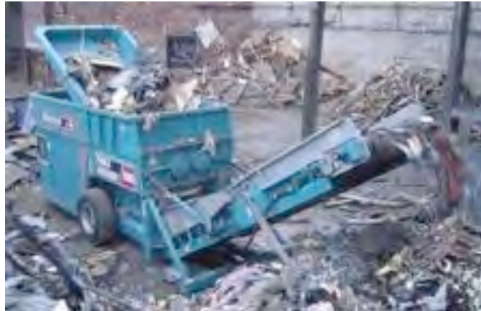
Figure 5.6-13 Solid waste shredder - Powershredder 1800 - by Powerscreen 42
