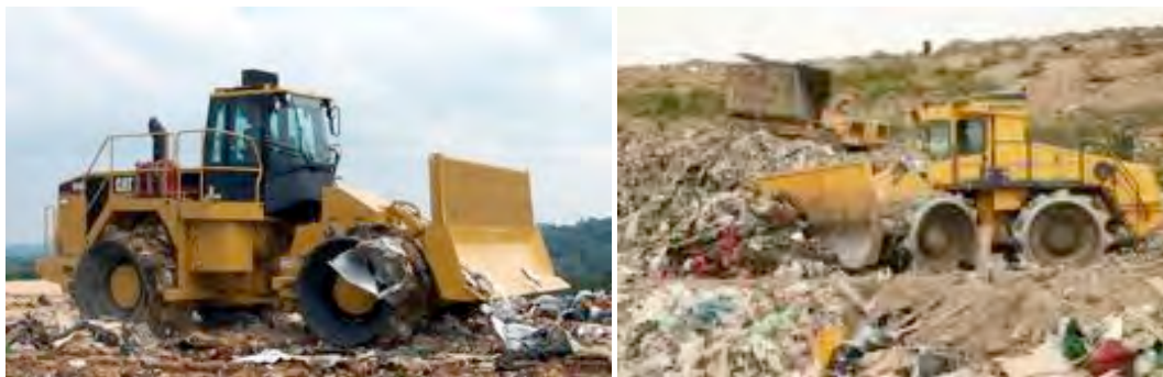
Figure 6.2-2 Various types of landfill compactors 45
