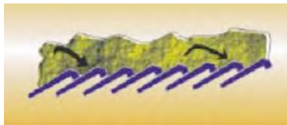
Figure 5.4-3: Principle of a reciprocating grate [Igelbüscher, 2005]
