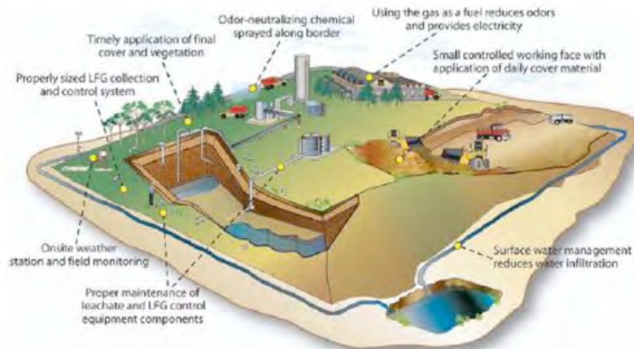
Figure 6.3-10 Methods to control odours at landfills [NAWMA, 2008]
