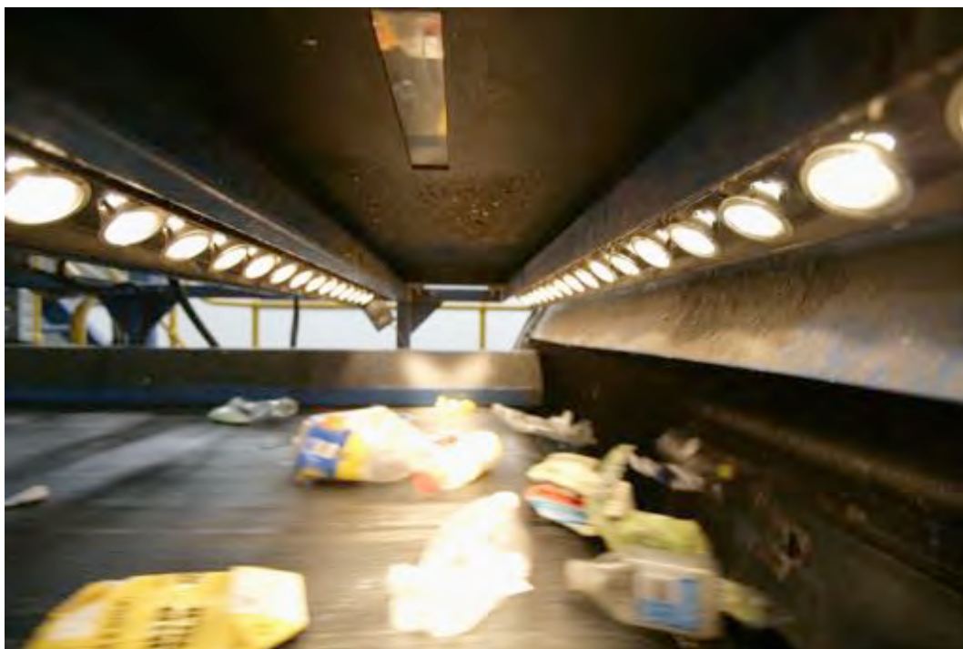
Figure 5.2-6: Optical sorting of plastics
