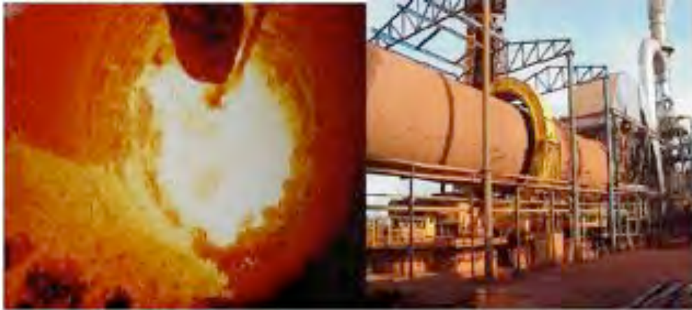
Figure 5.4-12 (left): Inside the rotary kiln
