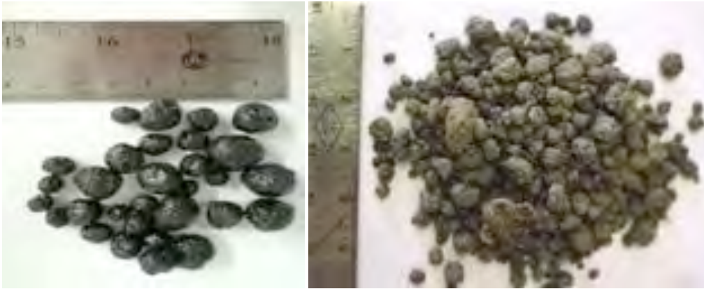
Figure 5.6-12 Terra-Bond™ waste encapsulation synthetic aggregates 41
